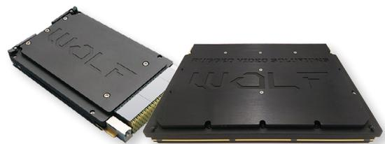
**The VPX3-4935 and VPX6-4955 feature NVIDIA Turing GPU technology and are designed for intense processing and AI in 3U HPEC systems**
