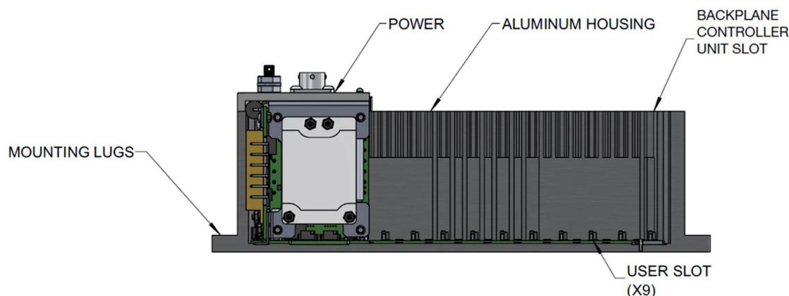
Figure 1: ADAUs consist of a chassis, power supply, controller, and user-selected modules
