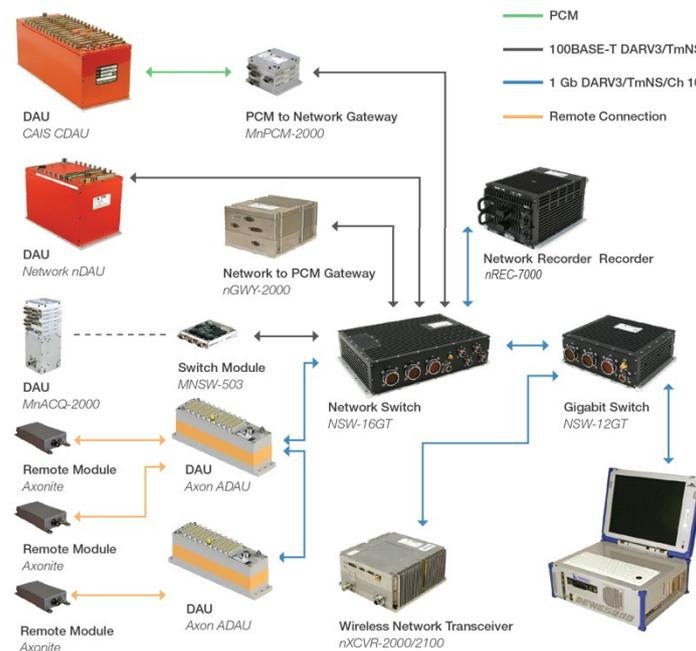
Figure 2: TTC DAU and ADAU Systems can be integrated seamlessly
