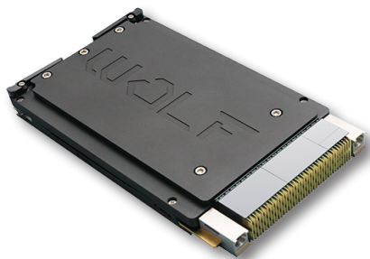
Figure 2: The VPX3-4935 3U OpenVPX module features NVIDIA Turing GPU technology and is designed for intense processing and AI in 3U HPEC systems.
