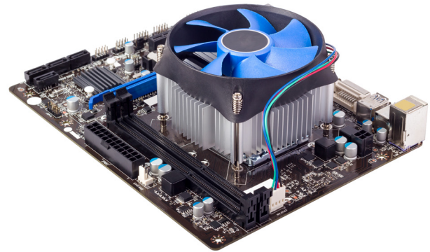
Figure 2: Heatsinks are effective for removing heat but are often impractical for ultra-compact systems due to their size
