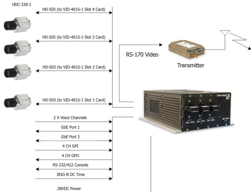
Figure 1: Camera networks usually include a recorder and the ability to telemeter data to a ground station.
