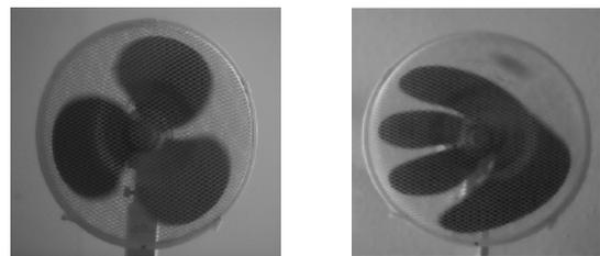
Figure 2: Global shutter (clear) and rolling shutter (distorted)
