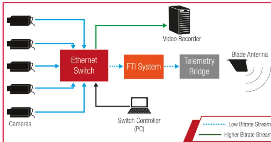
Figure 4: Dual compression on FTI cameras
