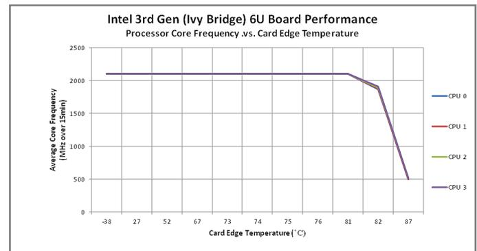
Figure 1: 6U VPX board performance with Intel's 3rd Gen Core i7 Processor Processor clock .vs. card edge temperature
