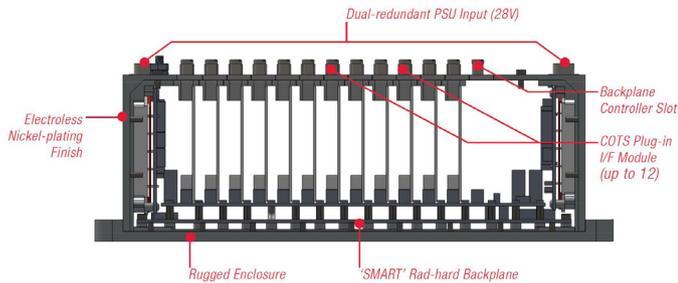
**Figure 5: The Smart Backplane design balances cost against risk**
