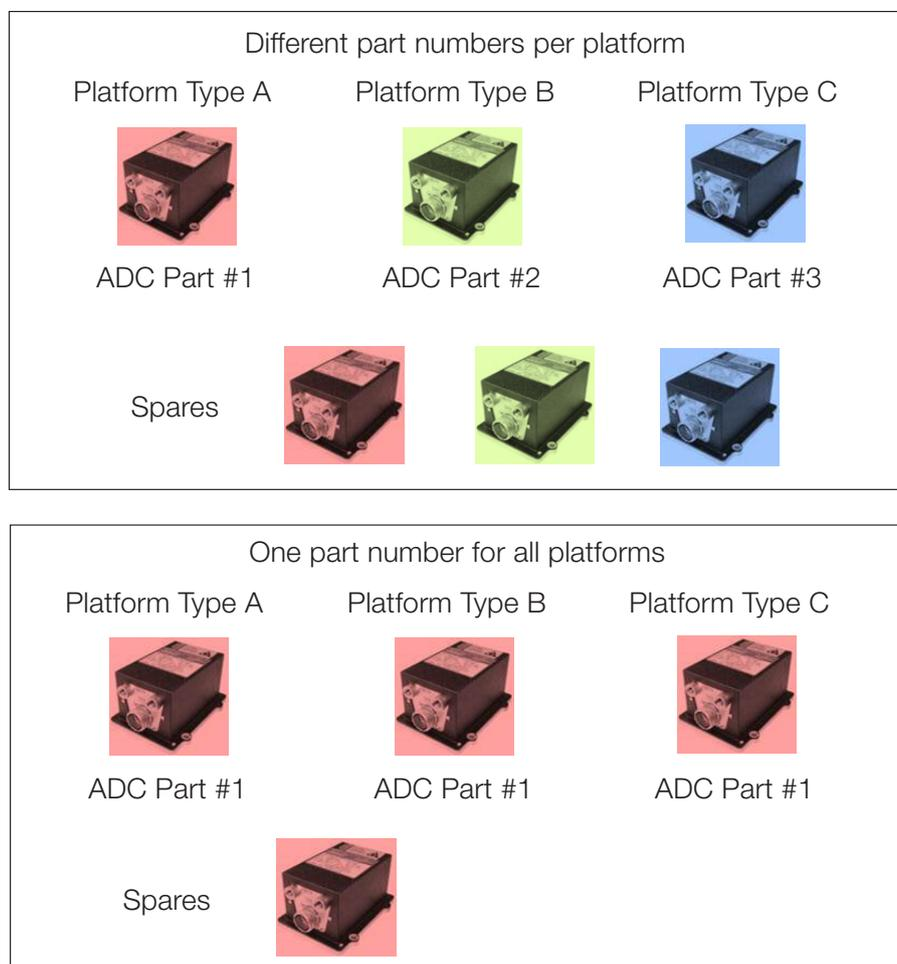
Figure 3. A bank of configurations stored within one ADC model eliminates the need to carry spares for all platform types
