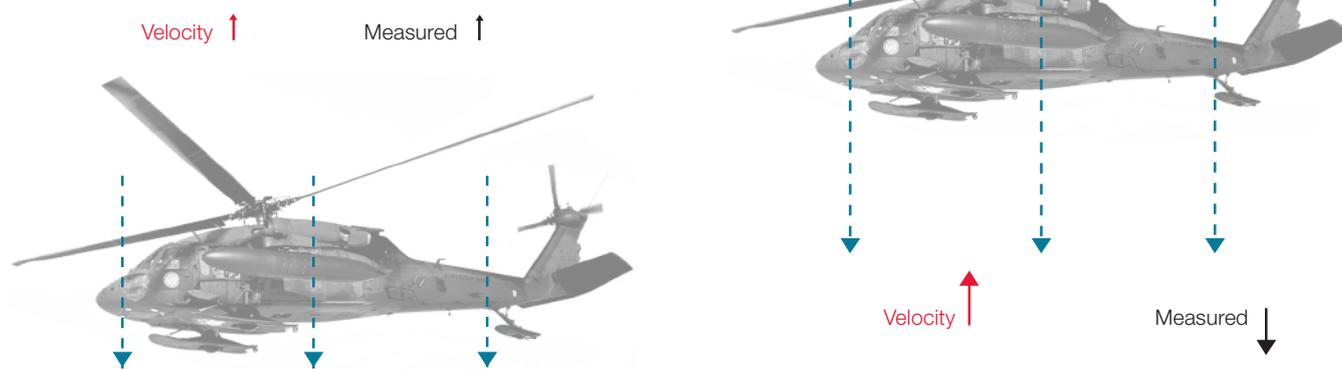
Figure 2. A rapid upward velocity caused a downwash to obscure the accurate measured velocity
