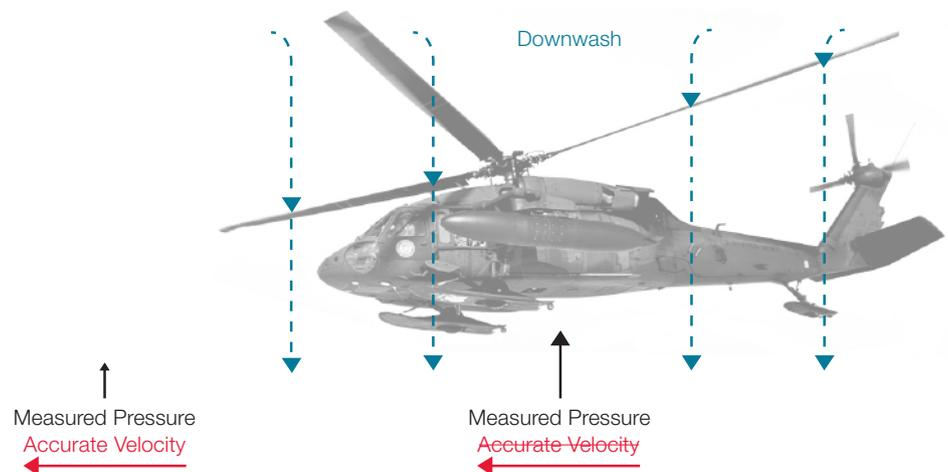
Figure 1. At low speeds, downwash interferes with accurate velocity readings
