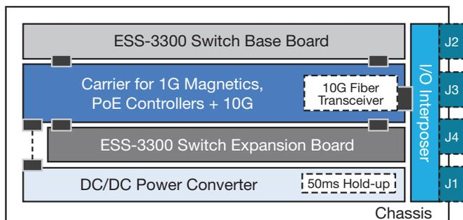
**Figure 3: DuraNET 3300 architecture block diagram**
