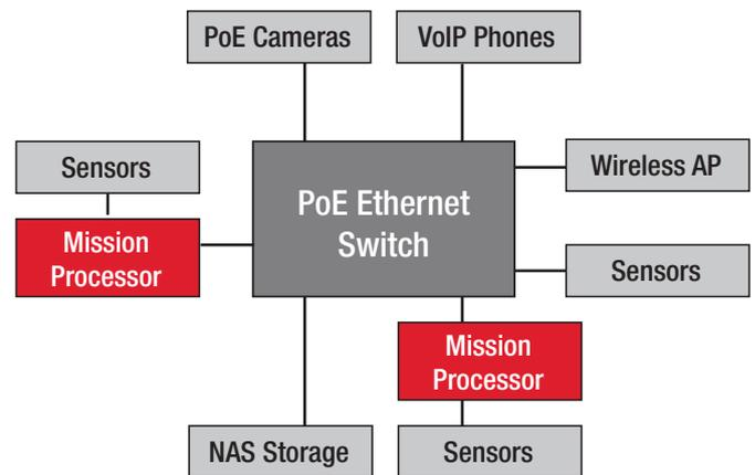
**Figure 2: C4ISR Ethernet LAN Backbone with PoE**
