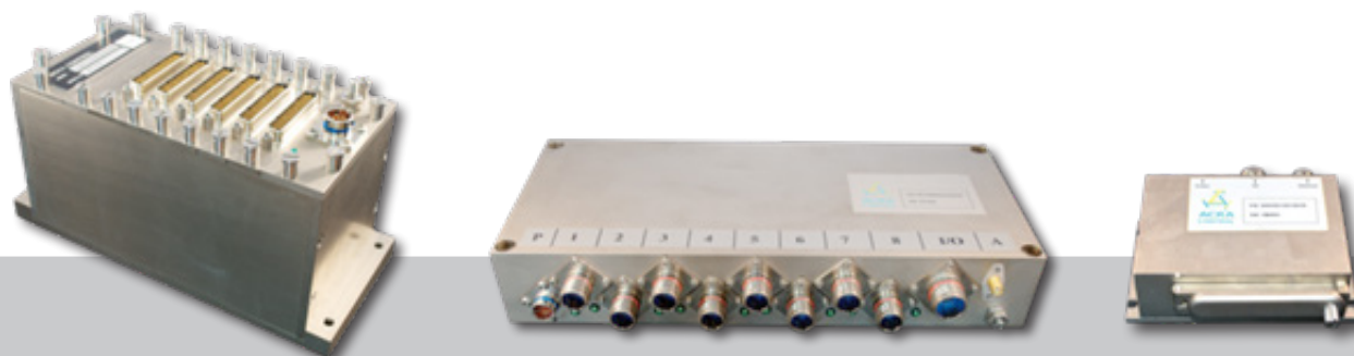
Figure 2: Rugged data handling spacecraft electronics
