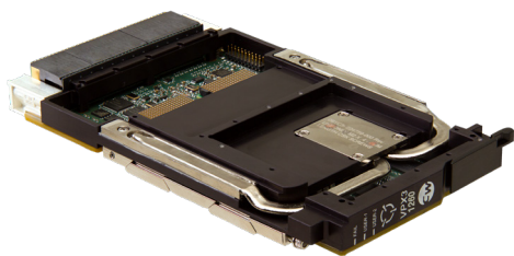
Figure 1: Curtiss-Wright's recently introduced VPX3-1260 SBC, powered by the new Intel Xeon® E-2176M (former codename "Coffee Lake") 8th Gen processor, is designed to take full advantage of hardware security features such as SGX and OS Guard.
