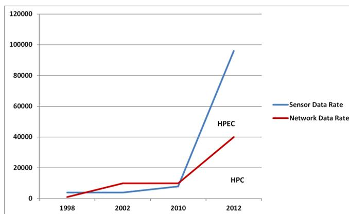
Figure 8: ADC to network technology gap
