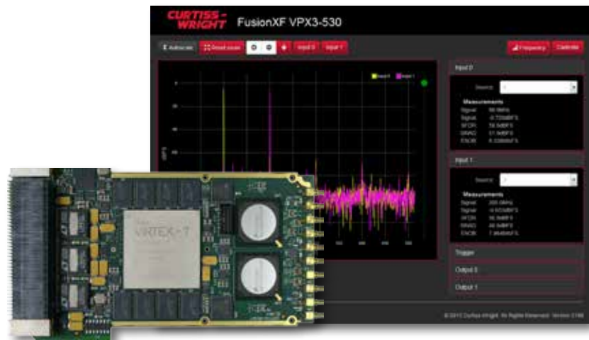
Figure 1: VPX3-530 digitizer/FPGA used for SDR
