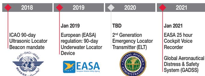
Figure 3: In the next few years, the regulations being introduced are aimed at more rapidly and reliably locating aircraft and their FDRs
