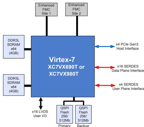
Figure 3: FPGA Memory & I/O
