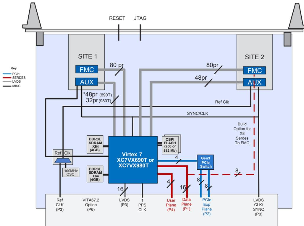
Figure 2: CHAMP-WB block diagram
