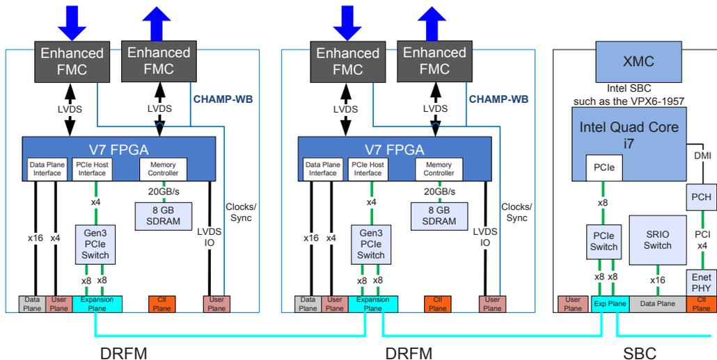
Figure 4: Diagram of 1957 with two CHAMP-WBs
