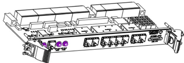
Figure 7: Line drawing of Rear Transition Module (RTM)
