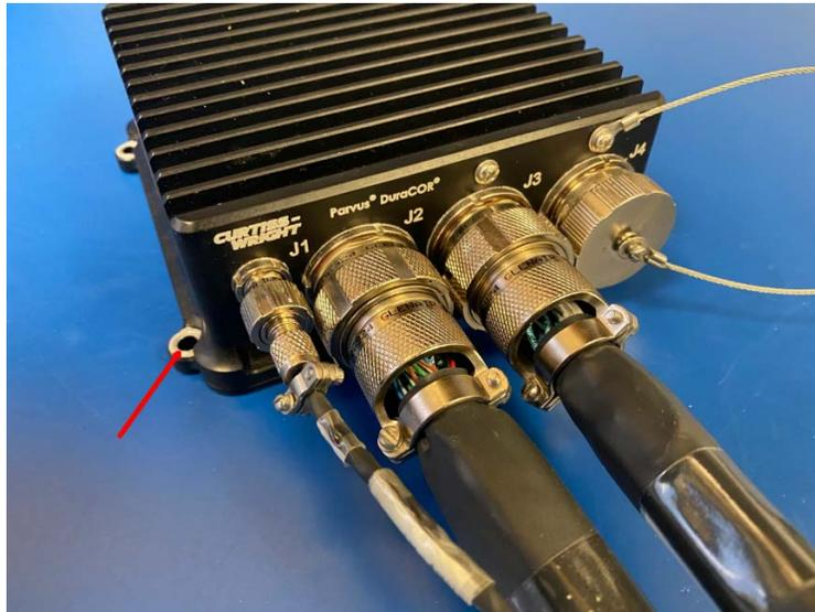
Figure 5) Recommended Chassis Ground for Double-Ended Cables.
