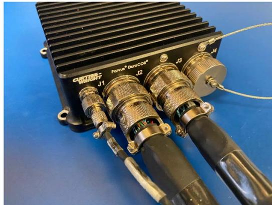
Figure 0) Sample product with 3 of 4 cable harnesses attached to 38999 connectors.
