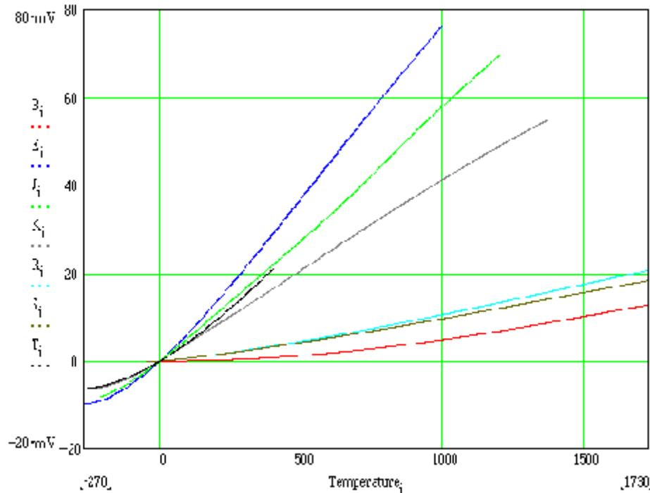
Figure 7-5: Voltage versus temperature for various types of thermocouples
