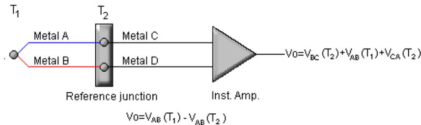
Figure 7-4: Summing the voltages about the thermocouple loop
