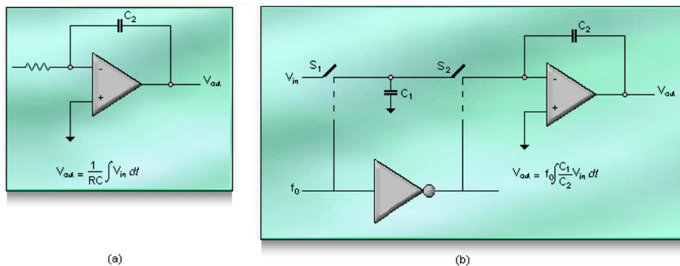
Figure 14-11: (a) Conventional integrator (b) Switched capacitor integrator
