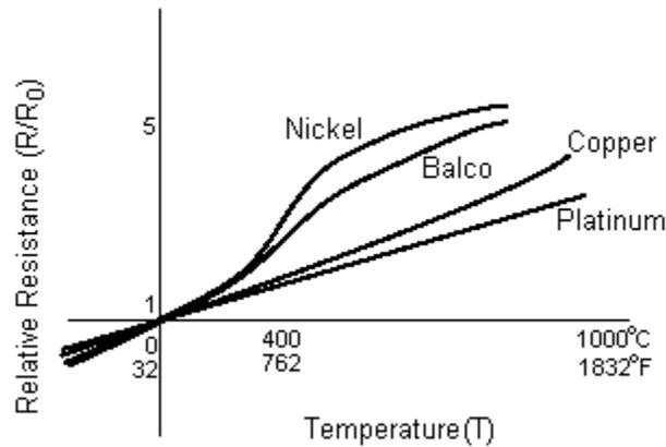
Figure 15-3: Resistance-Temperature relationship for some RTD materials
