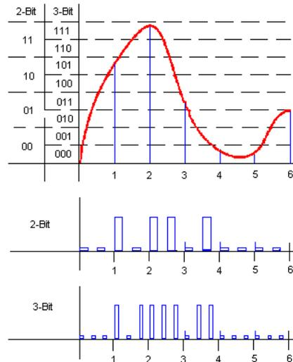
Figure 16-4: Pulse code modulation
