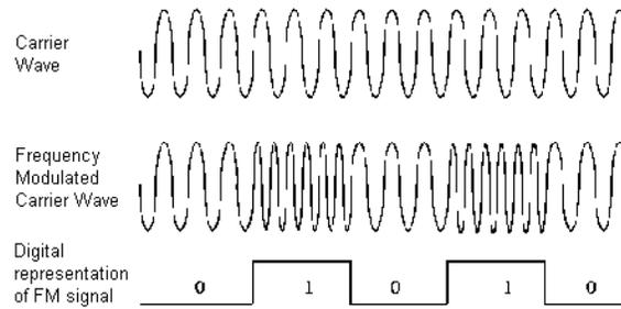
Figure 16-2: Frequency Modulation
