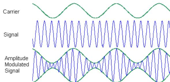
*Figure 16-1: Amplitude Modulation*
