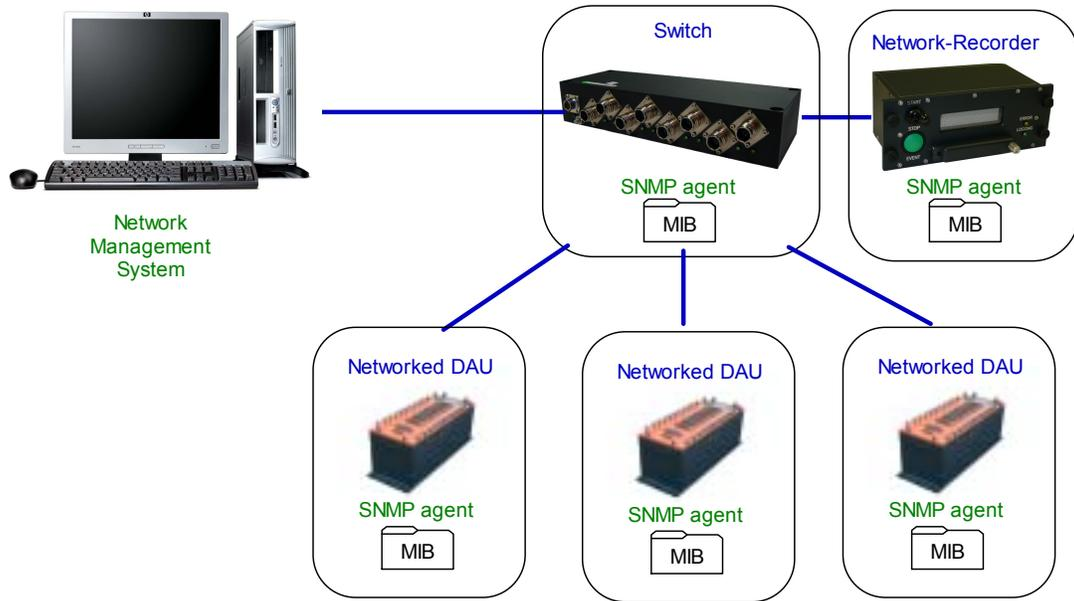
Figure 32-1: An SNMP-managed network
