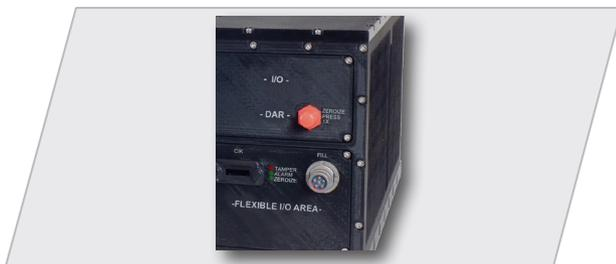
Figure 2: Flexible I/O and Type 1 Encryption
