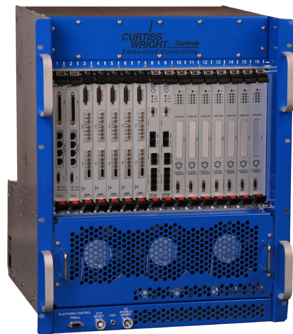
Figure 1: Curtiss-Wright HPEC system based on OpenVPX CEN16 backplane with SRIO-based CPU, FPGA and fabric switch modules.
