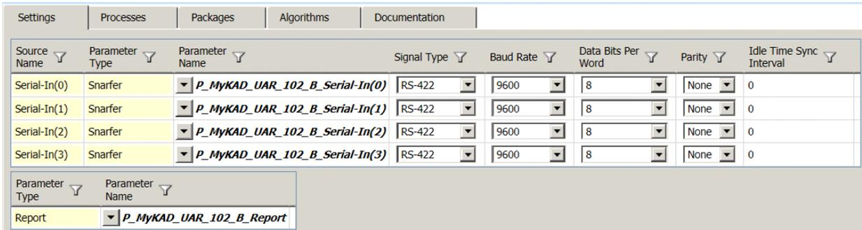
Figure 35-22: Snarfer parameters set using DAS Studio 3
