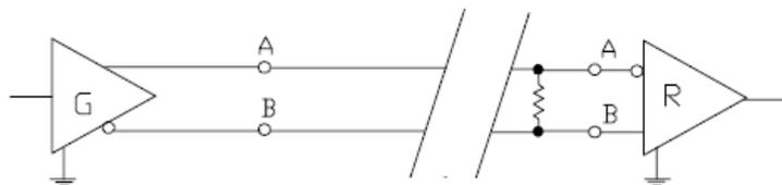
Figure 35-2: Termination differential input
