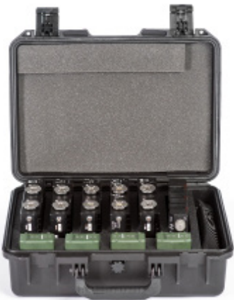
Custom case with 5x PacStar 400-Series modules, encryptor, tactical radio batteries and accessory bag
