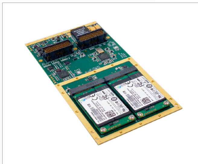
Figure 1: Curtiss-Wright XMC-554C COTS Mezzanine Memory Board
