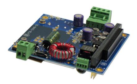
**FUNCTION:** Isolated PC/104 DC-DC Converter Vehicle Power Supply
