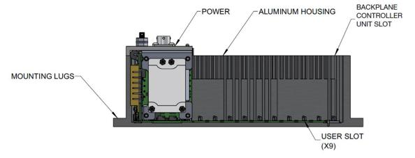
Figure 1: ADAUs consist of a chassis, power supply, controller, and user-selected modules
