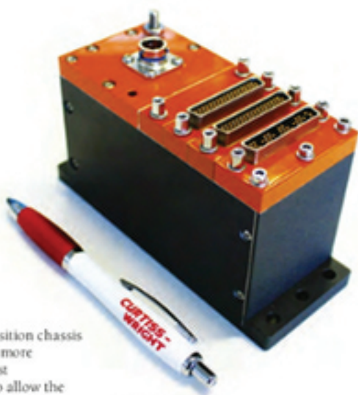
ABOVE: Miniature DAU chassis designed to enable closer location to an aircraft's sensors for FTI
