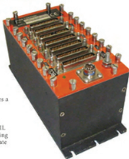
ABOVE: Curtiss-Wright's Acra KAM-500 is a COTS-based data-acquisition unit (DAU) designed for FTI applications
