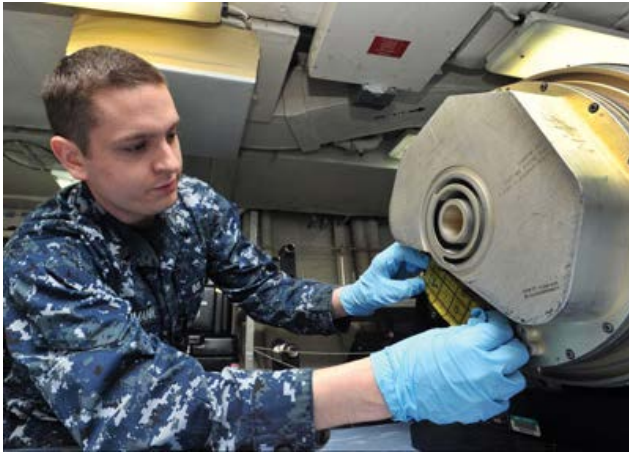
A Navy technician performs maintenance on an aircraft electro-optical sensor unit from a Navy attack aircraft. This sensor helps fighter-bombers drop precision bombs.
