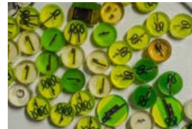
Micro-sections for electronics testing
