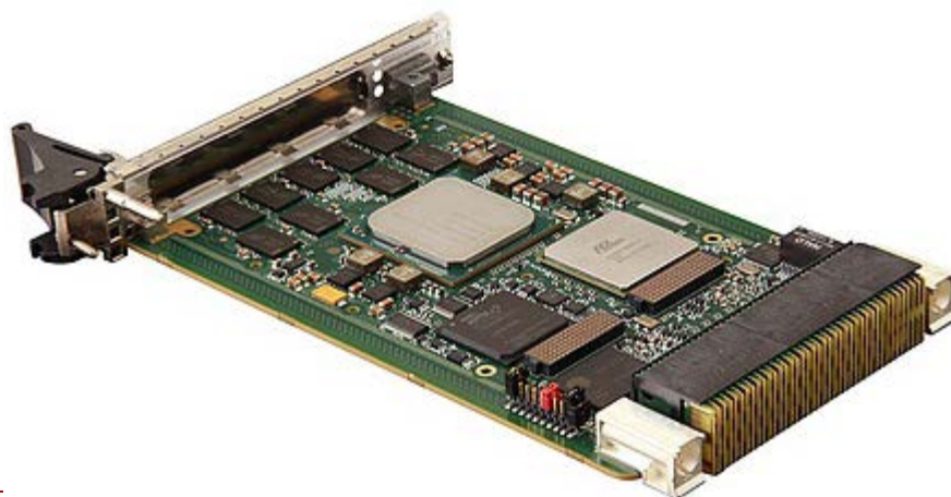
Figure 2: Curtiss-Wright's 3U OpenVPX CHAMP-XD1 is a SWaP-optimized DSP engine module that leverages the performance specs of Intel's Xeon processor D architecture for EW applications.
