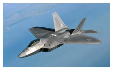
The Lockheed Martin F-22 Raptor is a 5th Generation fighter incorporating stealth shaping and radar-absorbent materials, as well as a passive radar detector with more than 30 antennas blended into the wings and fuselage for all-round coverage.
