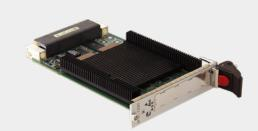
VPX3-1220 3U VPX 7th Gen Intel Xeon<sup>®</sup> Single Board Computer
