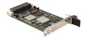
CHAMP-XD1 High-Performance Processor Card with Intel Xeon® D 8-Core D-1539 or 12-Core D-1559 processor
