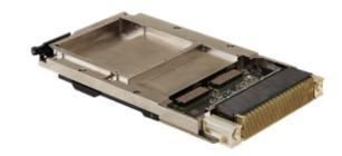
CHAMP-XD1S High-Performance Processor Card with Intel Xeon D 12-Core D-1559 processor
