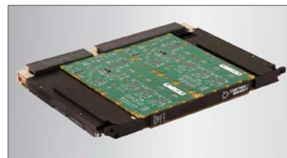
Figure 1 | The VPX6-195 single-board computer (SBC) offers two fully independent processor nodes on one 6U VPX board. The board's SBC nodes are isolated from one another so that failure in one does not conversely affect the other.
