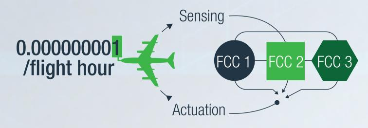
To protect against common mode failures, a fully fault tolerant system incorporates redundancy with dissimilar processor architectures, software and applications.
