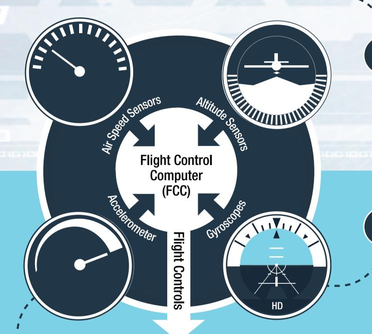
Most DAL A systems rely on data from multiple systems to calculate outputs.
