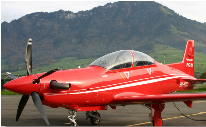
Figure 1: Pilatus PC-21: a single-turboprop, monoplane advanced trainer
