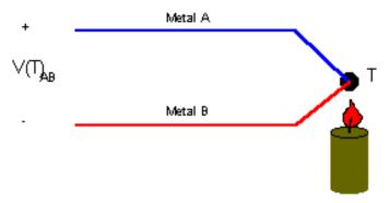
Figure 7-1: The Seebeck (thermoelectric) voltage
