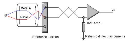
Figure 7-6: Twisting and shielding and return paths for amplifier bias currents
