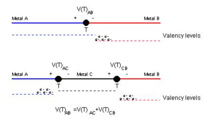
Figure 7-2: An illustration of the Law of Intermediate Metals
