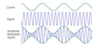
Figure 16-1: Amplitude Modulation
