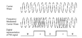
Figure 16-2: Frequency Modulation
