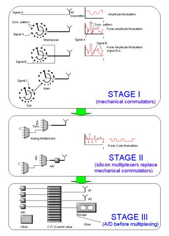
Figure 16-3: The evolution of communication technology
