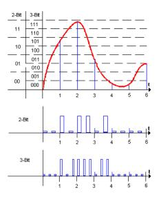
Figure 16-4: Pulse code modulation
