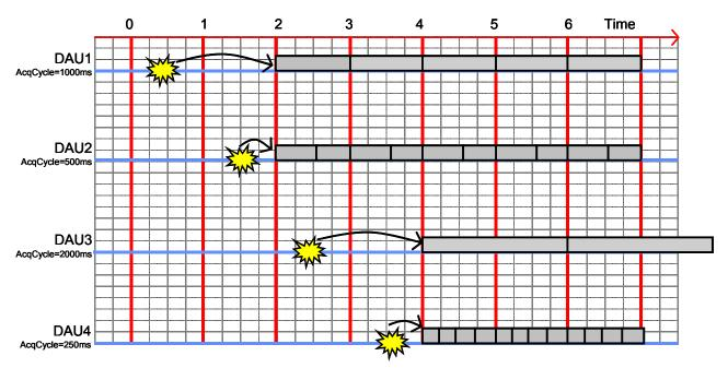
Figure 28-4: DAU acquisition cycles after synchronization
