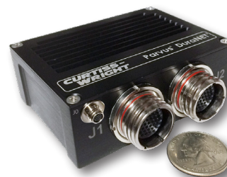
Parvus DuraNET 20-11 8-port Gigabit Ethernet switch
