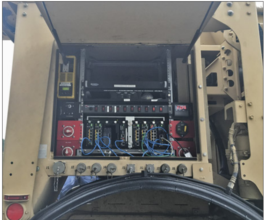
PacStar 400-Series Network Package on Joint Light Tactical Vehicle (JLTV)
