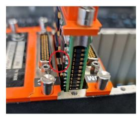
It is recommended that care should be taken when attempting to insert/extract the KAM/MEM/113 module to/from the chassis slot.
