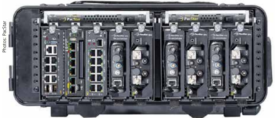
The PacStar Modular Radio Center (MRC) integrates SCI's TOCNET-G4 UVMS to bridge modern and legacy radio networks with industry-standard IP networks.
