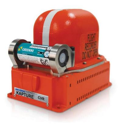
Universal Avionics foresees the ability to collect CVR and FDR data on a continuous basis for real-time analysis. Credit: Universal Avionics
