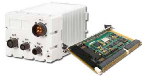
Figure 1 | Curtiss-Wright Controls Defense Solutions' MPMC-9335 3U VPX Mission Computer and its VPX6-187 6U VPX SBC are examples of FACE Candidate Hardware that can host FACE Candidate Software.
