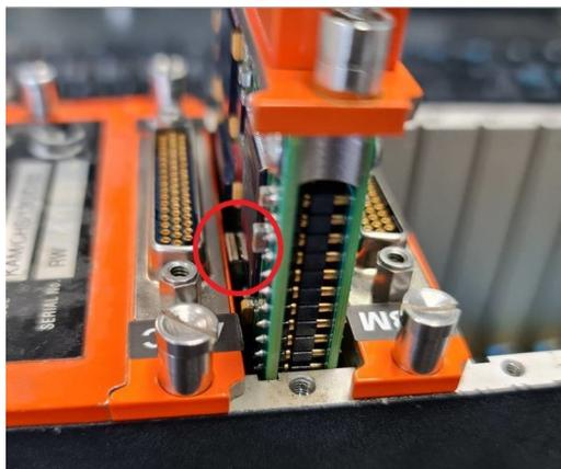
It is recommended that care should be taken when attempting to insert/extract the KAM/MEM/113 module to/from the chassis slot.
